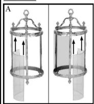
A) Coming up from the open bottom, slide the first glass panel up between the uprights with the clips. First fitting it into the grooves at the top and then the bottom.
